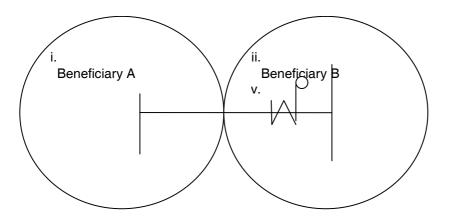
Case - 2: Interconnecting line owned by Beneficiary - B Metering point: Substation of Beneficiary-A
