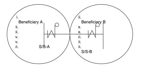
Net VArh exported from S/S-A, while voltage < 97% = X1Net VArh exported from S/S-A, while voltage > 103% = X2Net VArh imported at S/S-B, while voltage < 97% = X3Net VArh imported at S/S-B, while voltage > 103% = X4
